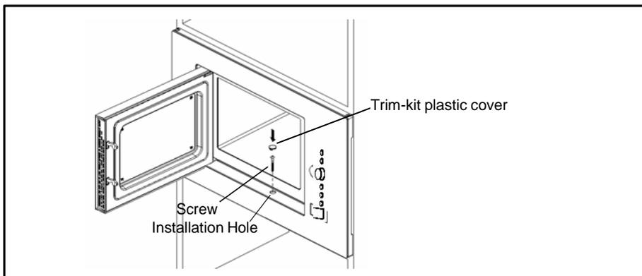
2. Open the door; fix the oven to the cabinet with **SCREW** at the **INSTALLATION HOLE** of **TRIM KIT**. Then fix the **TRIM-KIT PLASTIC COVER** to the **INSTALLATION HOLE**.
