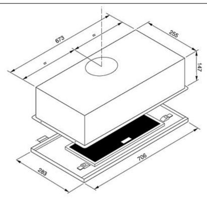
This unit must be installed to the underneath cupboard where the following area is recessed / setback (285mm x 710mm) by 40mm deep
