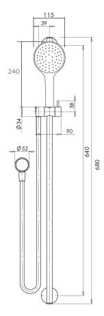
Complete slide rail length 680mm, adjustable bracket with single-jet handshower with rubber nozzles for easy cleaning and generous luxurious spray, 1500mm metallic flexible hose and wall union.
