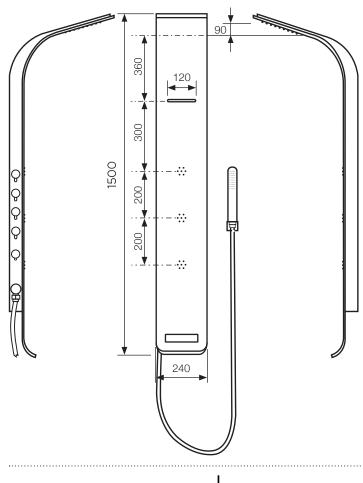
The Synergii shower panel is created from aluminum alloy with durable stainless steel hoses and brass bodies for the body jets.
