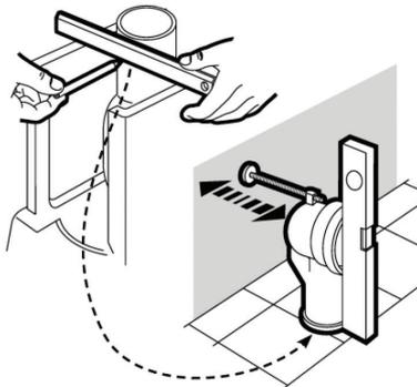
For **S Trap installation**, cut horizontal pipe to required length and fit seal. Attach wall fixing kit to elbow, push elbow into the pan collar and adjust to correct height. Fix to wall and adjust to ensure the elbow is vertical.
