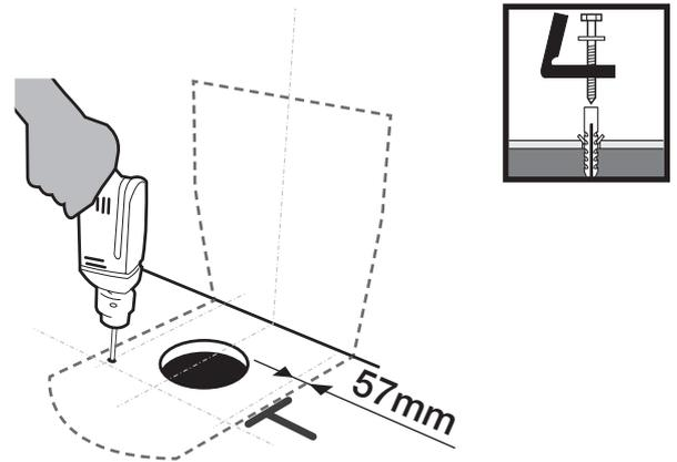
Remove pan, drill holes for fixing bolts and attach brackets.
