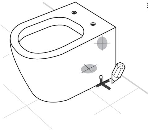
Place the pan in position ensuring it is centred in accordance with the centre line of the outlet. Mark location of pan fixing bolts.
