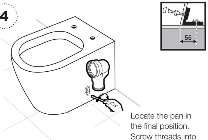
Locate the pan in the final position. Screw threads into floor mount brackets.
