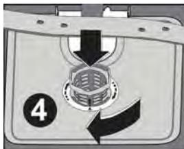
Pull and remove the metal/plastic filter. **3** Then pull the coarse filter out of the micro filter. **2** Rinse it with lots of water under the tap. Refit the metal/plastic filter. Insert the coarse filter into the micro filter in a way that the marks will correspond to one another. Attach micro filter into the metal/plastic filter and turn to the direction of arrow and it is locked when the direction of arrow and it is locked when the arrow on micro filter can be seen from across. **4**
