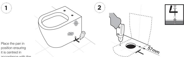
accordance with the centre line of the outlet. Mark location of pan fixing bolts.
