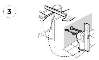
For **S Trap installation**, cut horizontal pipe to required length and fit seal. Attach wall fixing kit to elbow, push elbow into the pan collar and adjust to correct height. Fix to wall and adjust to ensure the elbow is vertical.
