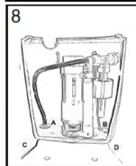
IF BACK INLET, SKIP THIS STEP. Remove cap from cistern plug A or B at base cistern. Connect flexible hose to cistern plug A or B depending on location of stop tap. Complete stop tap connection to underside of cistem plug C or D Fill cistern and ensure correct water
