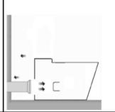
7 Place rubber seal into pan recess.( DO NOT USE SEALANT)
